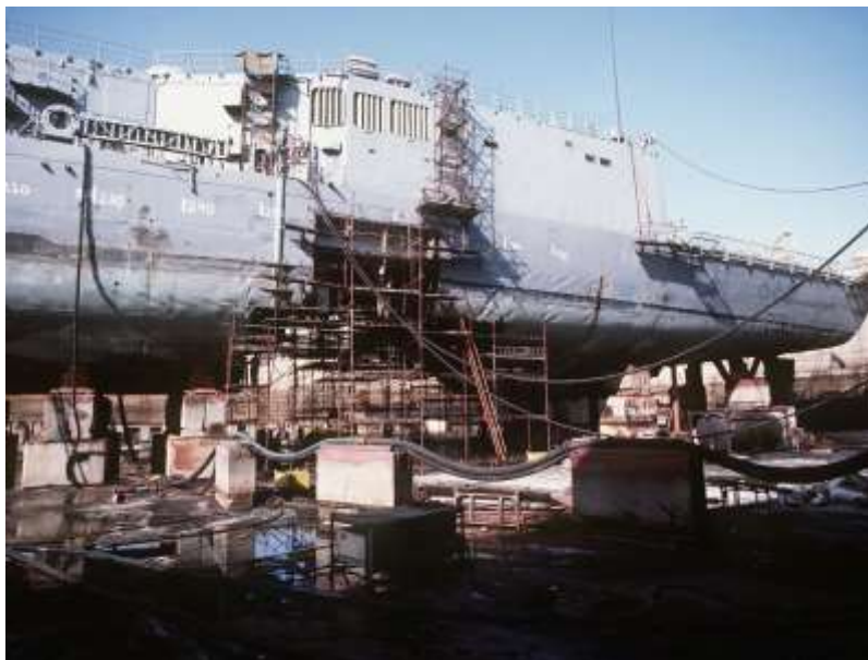
The frigate's hull was ruptured by the Iranian mine. The frigate was drydocked for repairs before it was sealifted back to the U.S.
